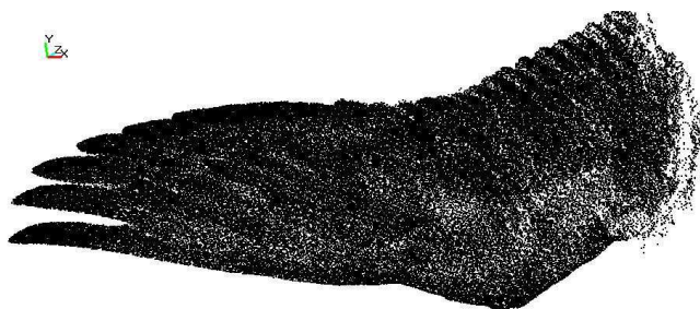
Figure 2. Data cloud of the surface of a seagull wing.
