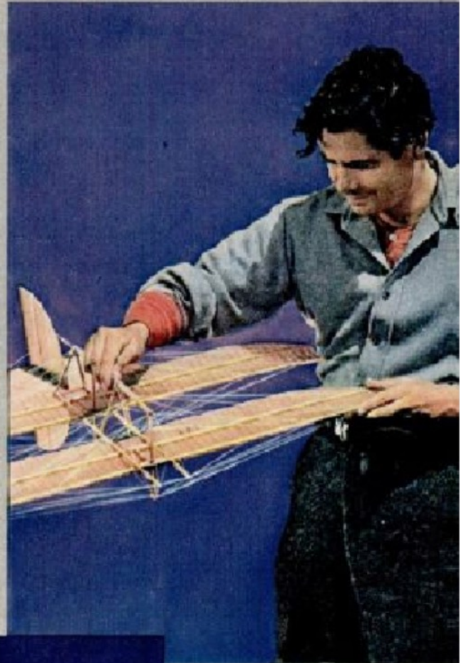
Tandem glider's wings were covered on top only. Its closely spaced ribs and wire bracing are evident in the model that Glenn Ford holds.
